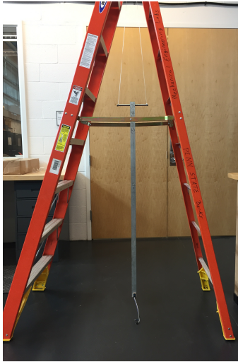
Fig. 1: Aluminum Beam Suspended from Ladder. The “T”-top of the beam was hung loosely with a loop of rope on each side attached to an eyehook at the top of the ladder. The bottom of the beam was suspended above the ground. An ADXL-335 accelerometer was affixed to the bottom of the beam and shown in more detail in Fig. 2.
